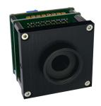
The APD development module from First Sensor is ideal for test runs in research and development as well as for integration into OEM LIDAR devices using the time-of-flight principle.
