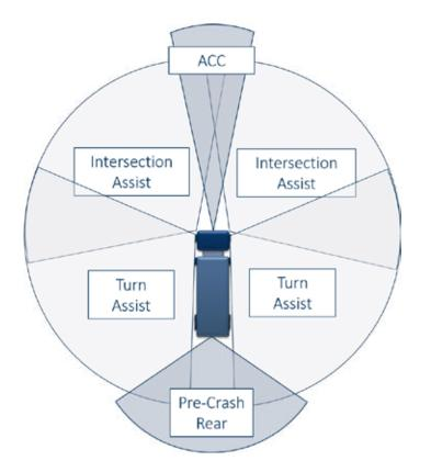
Due to its high angular resolution LIDAR is ideally suited for detection and classification of various objects (e.g. people, cyclists, animals, small object) in complex traffic situations. Sensor fusion with LIDAR data can dramatically increase the reliability of autonomous driving vehicles.
