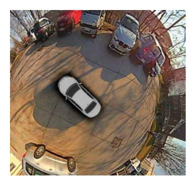
The Area View application is the latest technology of driver assistance systems coupled with long-term automotive camera design know-how. Designed to increase safety and comfort driving using several ADAS functionalities from 360° area view up to object recognition and its derivations, it supports the principle of accident avoidance. It meets the rising demand for an embedded and robust system for automotive, industrial and safety markets.
