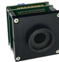
Receiver module with APD-Array, HV, TIA, MUX, Timing discriminator
