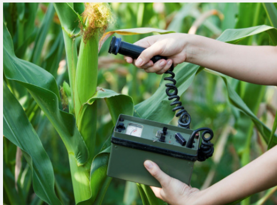
Figure 3: Radiation monitoring with conventional Geiger counter
